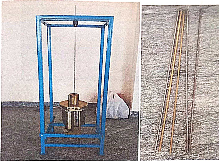
Figure 5.1 Damped torsional vibration tester and shaft materials
